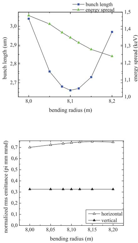
Figure 2: Simulated bunch length and energy spread (top) as well as horizontal and vertical normalized rms emittance (bottom) after the second bunch compressor as a function of its bending radius. The phase of the cavities is fixed.
