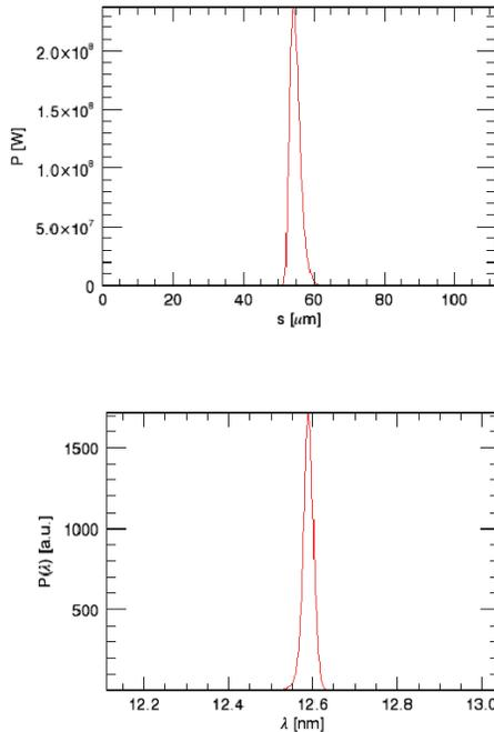
Figure 3: Simulated longitudinal SASE pulse distribution (top) and SASE spectrum (bottom) at the end of the FLASH undulators.
