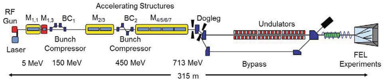
Figure 1: Schematic layout of FLASH (not to scale), including the beam energies used for the start-to-end simulation discussed in this paper. Generally, beam energies up to 1.25 GeV can be reached at FLASH.
