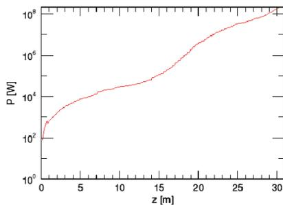
Figure 4: SASE radiation power vs. distance along the undulator.
