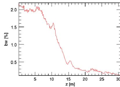
Figure 5: Bandwidth of the simulated SASE pulse.
