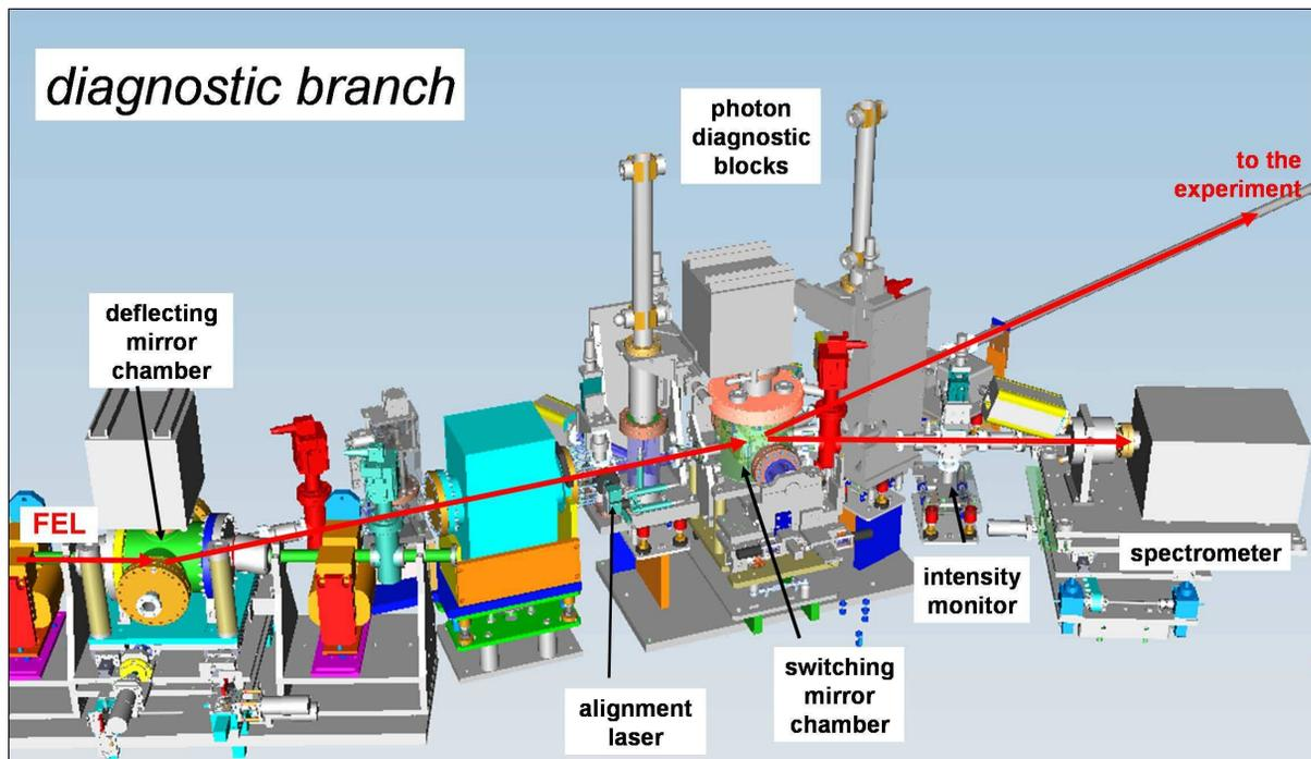
Figure 2: Layout of the photon beam line inside the FLASH tunnel. While the electron beam pass through a magnetic chicane the FEL radiation is deflected by the first three mirrors, then passes through the first diagnostic unit with YAG screen and different apertures. After that a further couple of mirror allows to send the photon beam either to the XUV-spectrometer or to the experimental hutch outside the tunnel.
