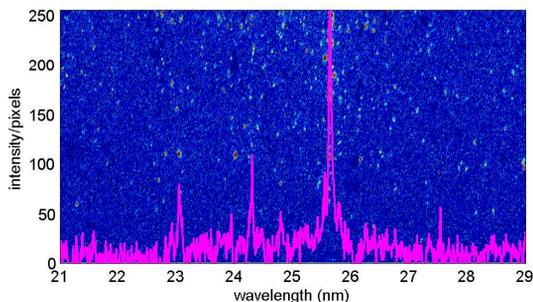
Figure 3: Spectrum of the plasma source.
