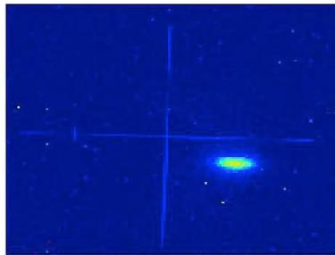
Figure 6: SASE radiation on the YAG screen in the first diagnostic block. The distance between the center and the first marker is 5 mm.
