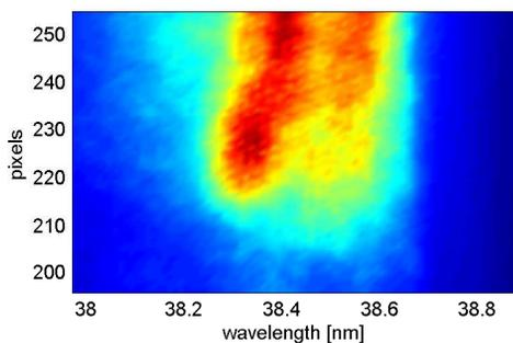
Figure 7: SASE single shot spectrum as recorded by the spectrometer with 100  $\mu\text{m}$  slits.
