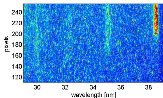
Figure 4: Spectrum of the HHG source as recorded by the spectrometer in the diagnostic branch. Exposure 10 s, slits  $500 \mu\text{m}$ .
