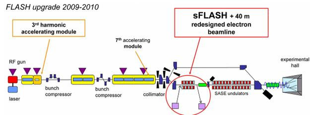
Figure 1: New layout of FLASH after the shutdown: a third harmonic cavity is installed before the first bunch compressor and the section between the collimator and the SASE undulators accommodates the components for the seeding experiment.
