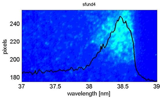
Figure 5: Spectrum of the spontaneous radiation from the last sFLASH undulator. Exposure 1 s, slits 500  $\mu\text{m}$ .
