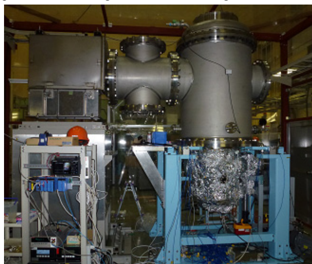
Figure 1: A photograph of the second DC-gun. The HVPS (left) is connected to the gun chamber (right).
