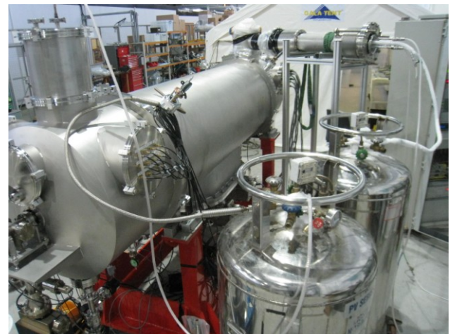
Figure 2: Fully assembled cryomodule undergoing Qualification tests.
