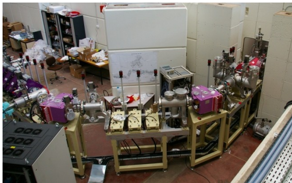
Fig. 3: Spiral 2 LEBT under construction at Saclay
