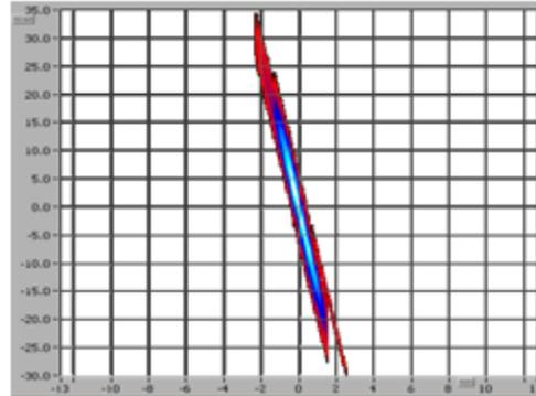
Figure 8: 2 mA H<sup>+</sup> beam emittance after the solenoids
