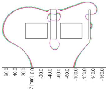
Figure 7: Optimized magnetic configuration and 87.5 mT ECR location
