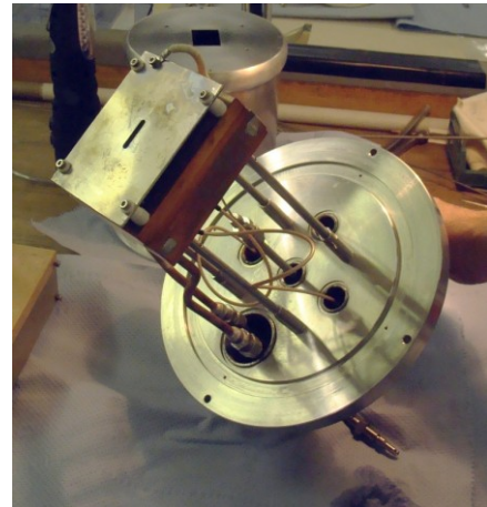
Figure 5: T-COMIC with up to three discharge and plug & play by respect to a filament source.
