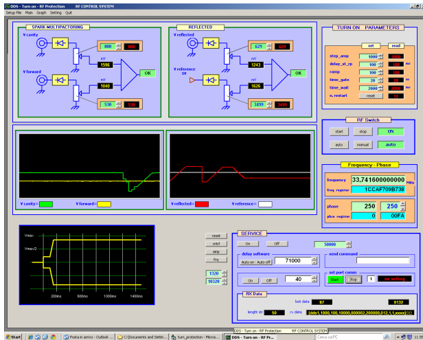
Figure 5: Low Level RF-Box control panel.
