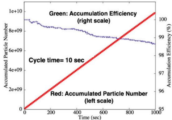
Figure 7: Increase of stacked antiproton number (red) and accumulation efficiency (green) for the moving barrier method.
