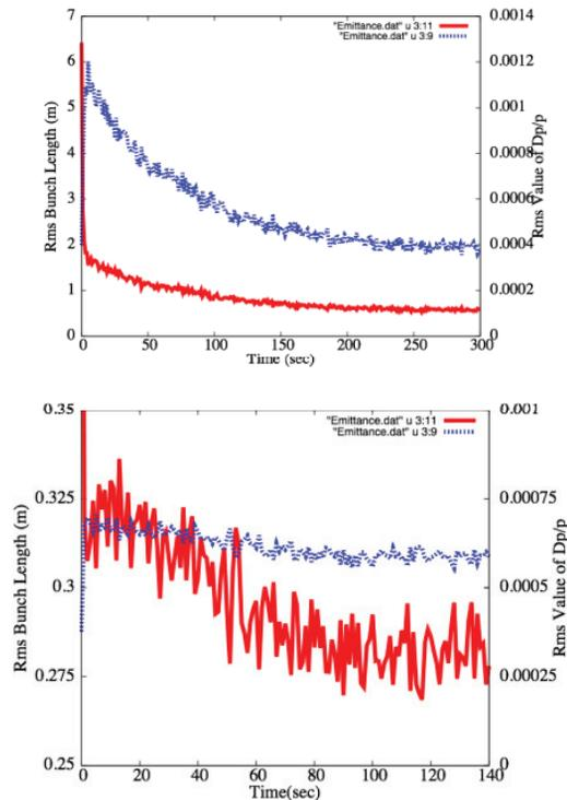
Figure 10: The evolution of bunch length (red) and  $\Delta p/p$  (blue) in the process of short bunch formation at the 1<sup>st</sup> step (top) and the 2<sup>nd</sup> step (bottom).
