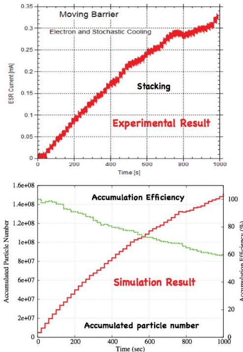
Figure 8: The experimental (top) and the simulation (bottom) results of the moving barrier operation. The red line in the bottom figure shows the accumulated particle number and the green line the accumulation efficiency.
