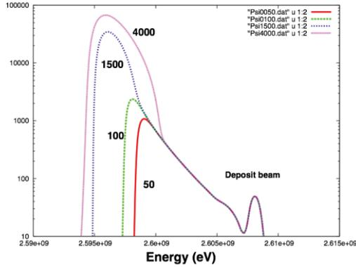
Figure 2: The simulated beam profile of 2.6 GeV anti-proton beam for different stacking numbers for the CERN AA. Cycle time is 5 sec and deposited particle number is  $1 \times 10^8$ .
