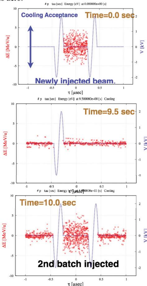
Figure 5: The particle distribution in the longitudinal phase space at time= 0 (top), 9.5 (middle) and 10 sec (2<sup>nd</sup> injection) (bottom) for the moving barrier method for the HESR. Barrier voltage (blue) and particles (red points).
