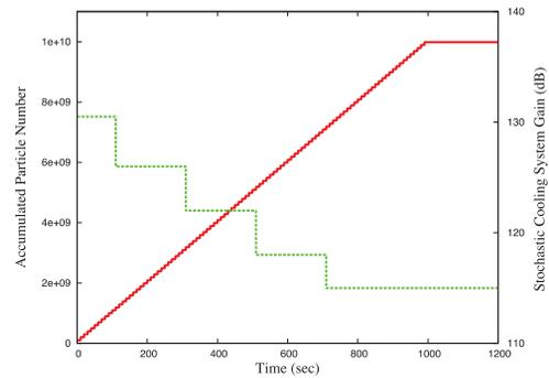
Figure 6: The accumulated particle number (red, left scale) and the electronic gain of the cooling system (green, right scale). Horizontal scale is time (sec).
