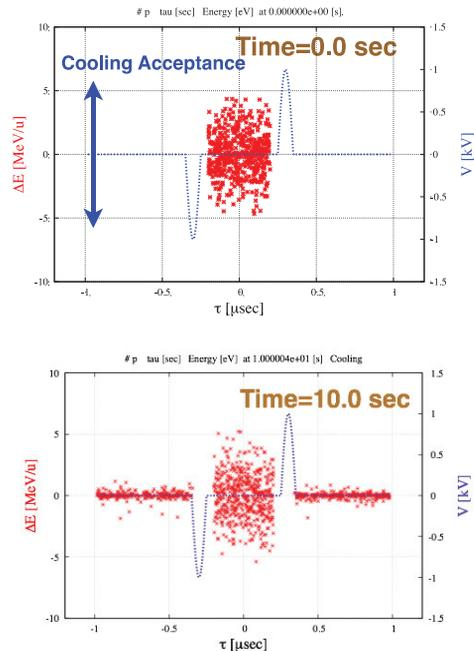
Figure 3: The particle distribution in the longitudinal phase space at time= 0 (top) sec and 10 sec (2<sup>nd</sup> injection) (bottom) for the fixed barrier method for HESR. Barrier voltage (blue) and particles (red points).
