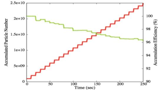
Figure 9: The increase of accumulated particle number (red) and accumulation efficiency (green) during 25 times injection. The cycle time is 10 sec.
