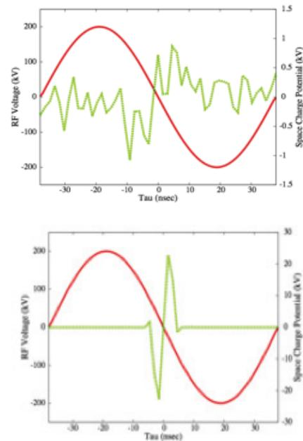
Figure 11: Comparison of external 200 kV RF (red) & space charge potential (green). From the top to the bottom, time is 1 and 100 sec, respectively. The ion number is  $1 \times 10^9$ /bunch.
