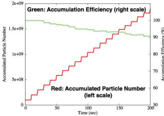
Figure 4: Increase of stacked antiproton number (red) and accumulation efficiency (green) at the fixed barrier method.
