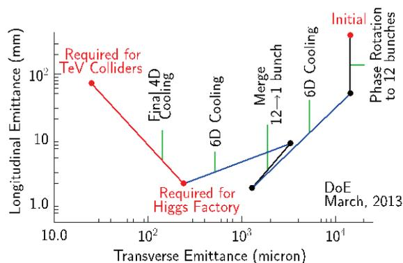
Figure 2: Emittance evolution along a 6D ionization cooling channel for a Muon Collider (MC). The entrance to the channel is the point at the upper right of the plot. The very small energy spread required for a Higgs Factory could be obtained by stopping at the bottom red point. Smaller transverse emittances, and hence higher luminosities for TeV-scale colliders, would require letting the cooling continue to the upper left red point.
