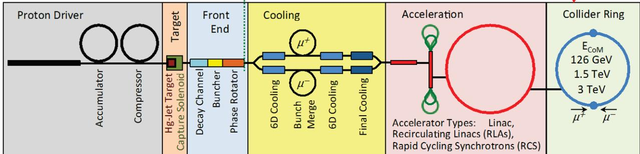
Figure 1: Block diagrams showing the principal elements of a Neutrino Factory (NF) and a Muon Collider (MC). In a dual-purpose facility, it is envisioned that the NF and MC will operate with a shared proton driver, target and front end.
