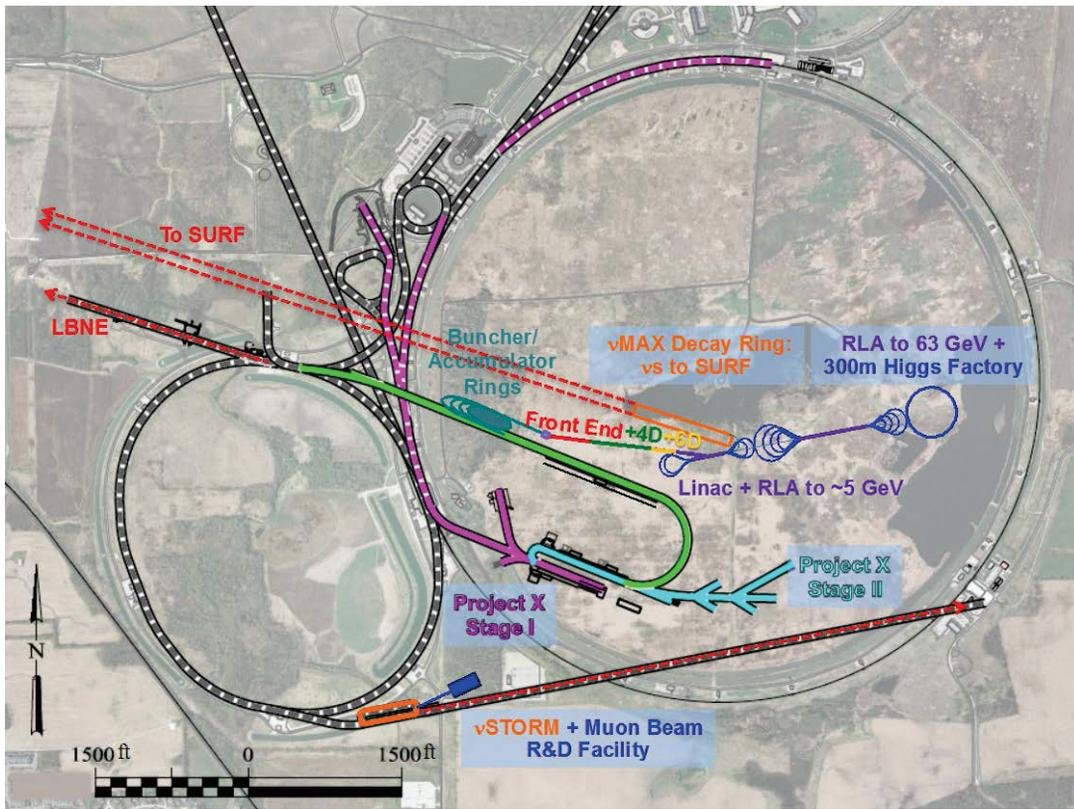
Figure 3: A staged facility, from vSTORM through the implementation of a Higgs Factory, on the Fermilab site. The second stage, implementation of the NuMAX Neutrino Factory capability, could be built on the foundation of the Project X Stage II CW Linac operating at 3 GeV proton energy.
