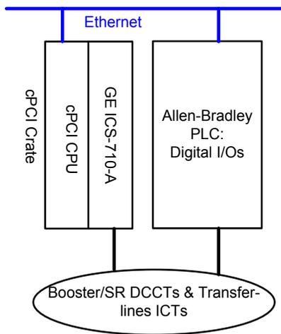
Figure 2: Overview of beam intensity measurement.
