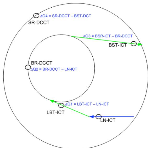
Figure 1: NLSLS-II beam intensity monitors and injection efficiency measurements.
