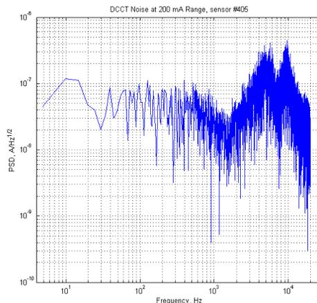
Figure 4: Bergoz NPCT spectral noise density.
