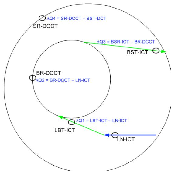
Figure 1: NSLS-II beam intensity monitors and injection efficiency measurements.
