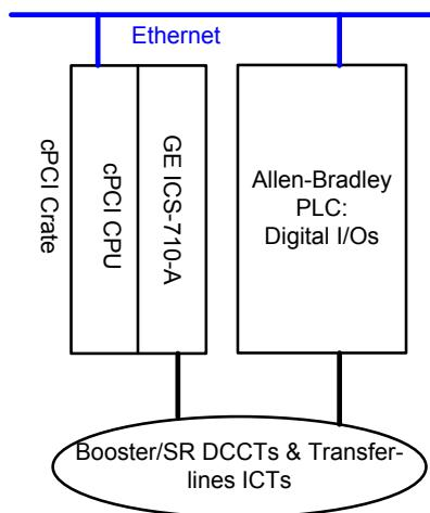
Figure 2: Overview of beam intensity measurement.
