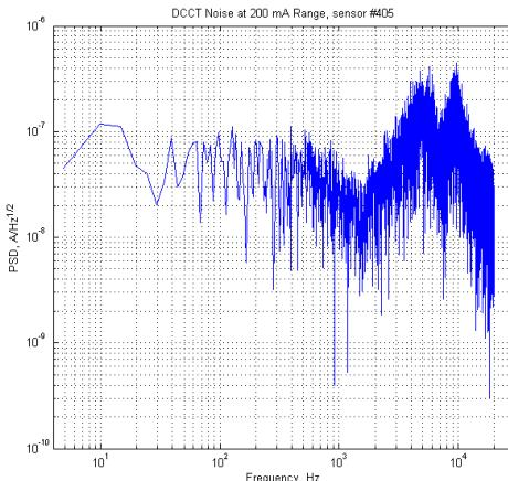
Figure 4: Bergoz NPCT spectral noise density.
