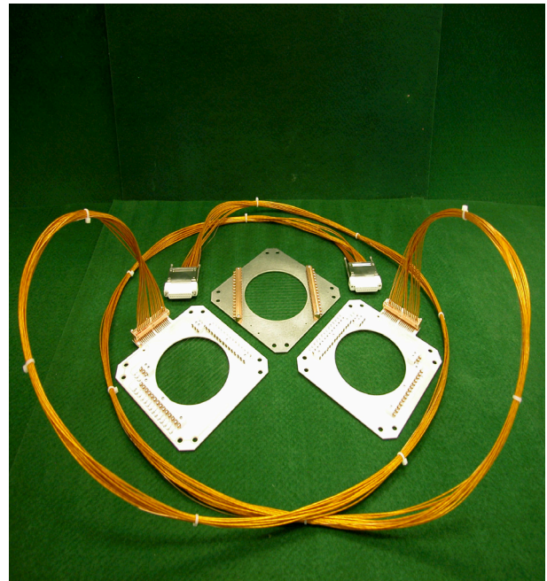
Figure 5: Three planes of 1L Harp with 0.079-mm SiC fibers attached using a collet style of clamp.
