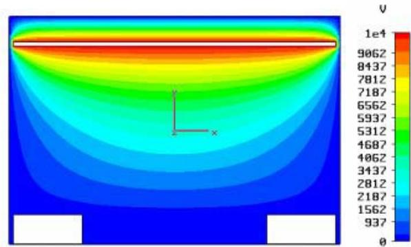
Figure 11: Transverse electrostatic potential distributions in the ISIS ring profile monitors.
