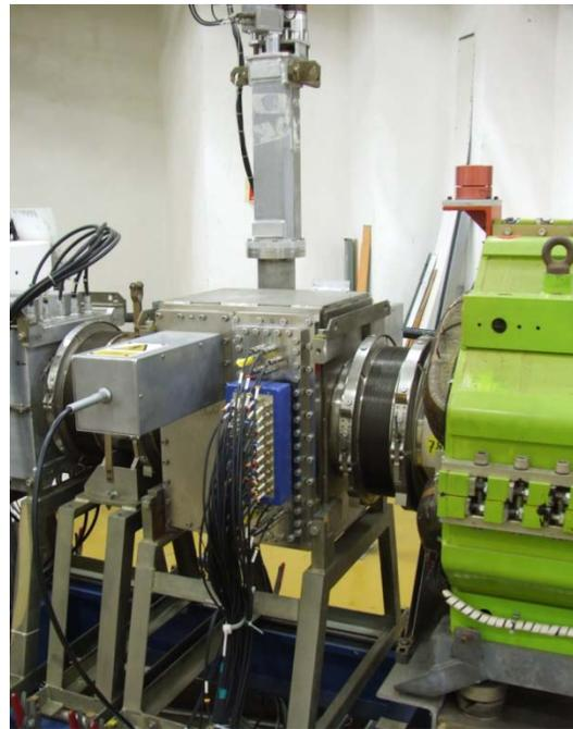
Figure 5: Second generation multi-channel profile monitor installed in the ISIS synchrotron. The motor drive of the SCPM can be seen diagonally opposite.
