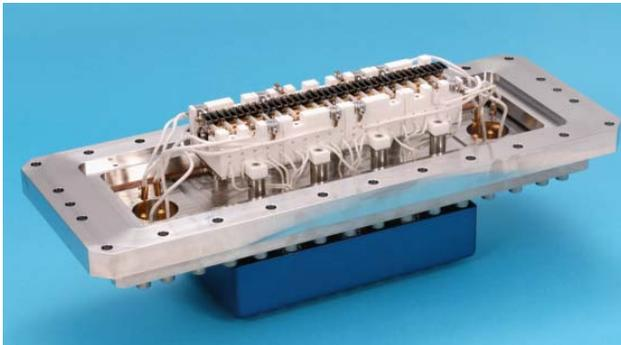
Figure 2: First generation multi-channel profile monitor using a (40) Channeltron array.
