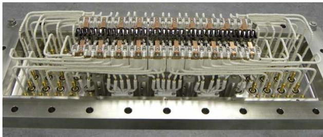
Figure 6: Third generation multi-channel profile monitor.
