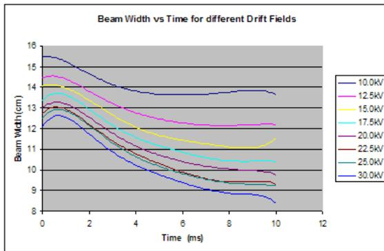
Figure 8: Measured beam width for different drift field voltages over the ISIS acceleration cycle.
