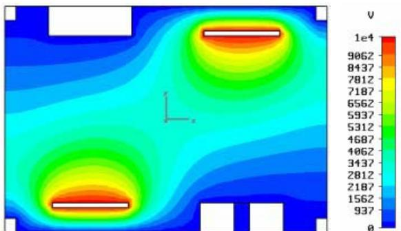
Figure 10: Longitudinal electrostatic potential distributions in the ISIS ring profile monitors.
