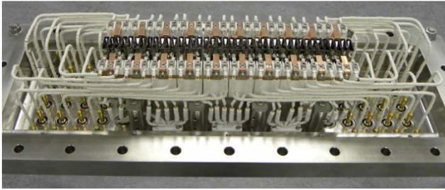
Figure 6: Third generation multi-channel profile monitor.
